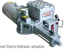
The self-contained Electro-Hydraulic actuators consist of control, hydraulic, and power modules incorporating a motor driven pump with a hydraulic cylinder. These actuators offer complete tailor-made solutions to a client's application needs such as emergency shutdown (ESD), on-off modulating control, and partial stroking tests with minimal effect on the process.
