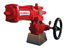
The compact FB declutchable gear override provides efficient, precise performance for quarter-turn manual override duties. The gearbox is specially designed to offer quick and simple operation of the highest torque valves when the air or power supply fails. High precision, selflocking gears provides safe, positive manual positioning and extend gearbox life.
