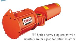
modulating duty, and can be provided with either symmetrical or canted torque output to suit the duty requirements of the valve. They have been certified to meet SIL 3, 4 ratings in accordance with IEC 61508/61511, which will support plant operations under safety instrumentation systems.
