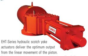
This is ideal for quarter-turn valve applications. The EHT actuator is smaller than other actuators offering similar torque outputs. which reduces the overall valve package envelop, allowing for a more compact design.
