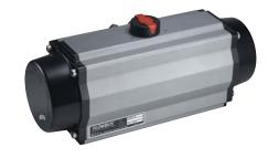
EPR-Series actautors feature a compact Rack & Pinion and modern Scotch Yoke mechanisms. The extruded aluminum body incorporates an advanced, hard anodizing treatment on the internal and external surfaces and the body can also be provided in a number of optional finishes including PTFE coated, electroless nickel plated, and a variety of polyester power coated colors for udrability incrase and corrosion protection.
